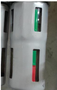
Figure 3: Service unit visuals to display acceptable and unacceptable oil levels.
