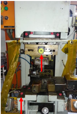
Figure 7: Colour coding of bolts to distinguish between adjustments for maintenance and production.
