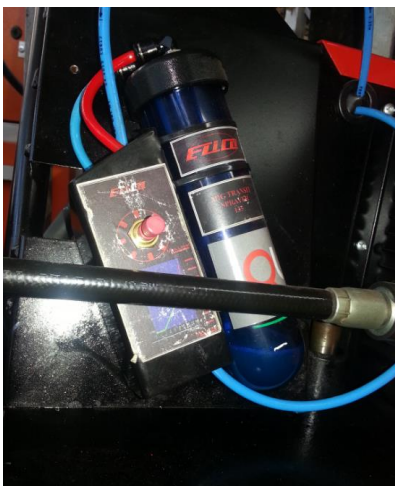
Figure 8: An anti-spatter device added to the Auto-Welder has reduced the frequency of cleaning the Auto-Welder gun nozzle.
