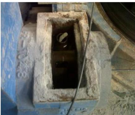
Figure 3: Identifying sources of contamination that leads to forced deterioration and breakdowns
