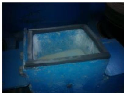
Figure 5: Rubber sealing strip added on all die boxes to seal with lid cover when the machine is running
