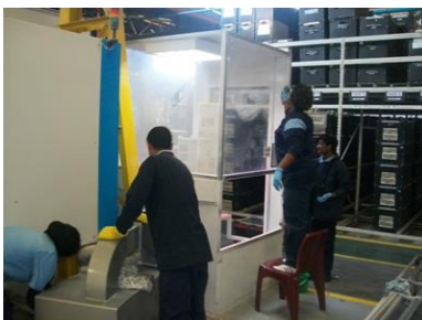
Figure 3: Operators cleaning their machines as part of step 1 Autonomous Maintenance with reference to their cleaning standards developed through the programme.
