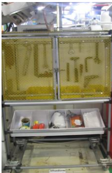
Figure 5: Tool cupboards cluttered with unneeded items. After, shadow board developed with all required tools and consumables.
