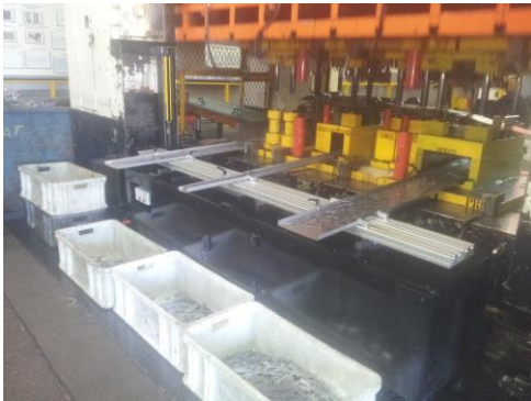
Figure 1 Scrap Shakers: The above figure shows the breakthrough development of a Scrap Shaker, this will eliminate the time stop to remove the off-cut pieces
